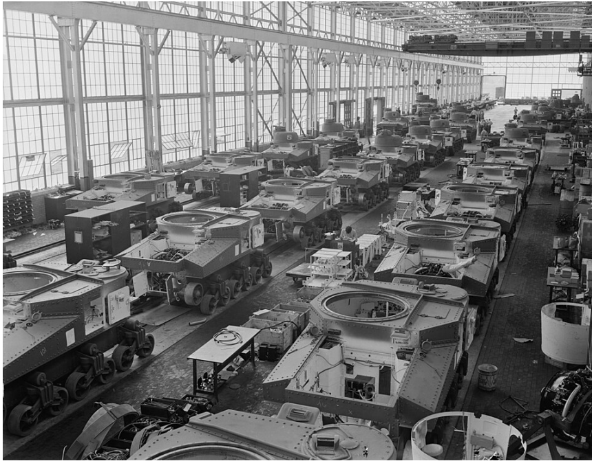
Figure 11: Tank manufacture (Chrysler). These are partially completed M-3 tanks, twenty-eight ton steel giants being turned out at the huge Chrysler tank arsenal in Detroit. The camera was directed toward the end of the three main assembly lines. Mass assembly methods developed in automobile manufacture are used. Note overhead cranes for heavy parts.
